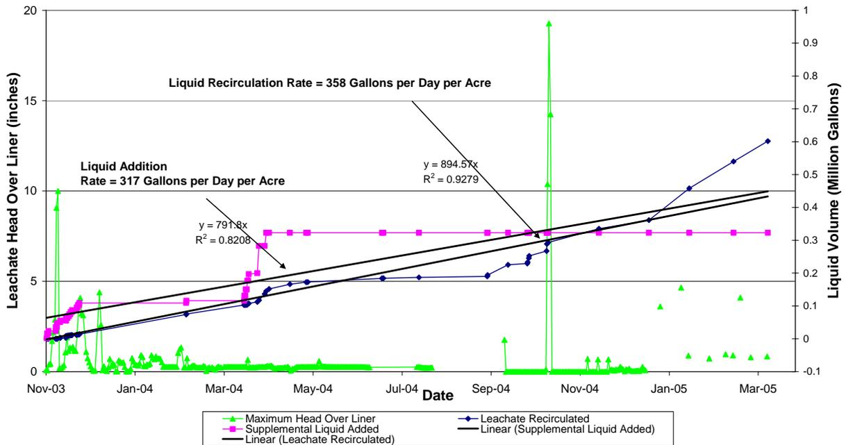
Note: In March 2004, one out of the two pressure transducers under the southeast cell began giving erratic readings that were not supported by pressure tube readings. In August 2004, both pressure transducers were removed and recalibrated. The one that was previously giving erratic readings was determined to have failed and removed from the system. In January 2005, the other sensor failed, thus maximum head over liner curve was created using pressure tube data.
