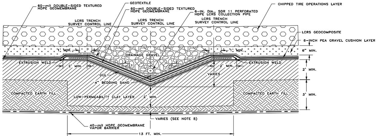
**Detail 4. Module D bottom liner and leachate collection trench cross-section**
