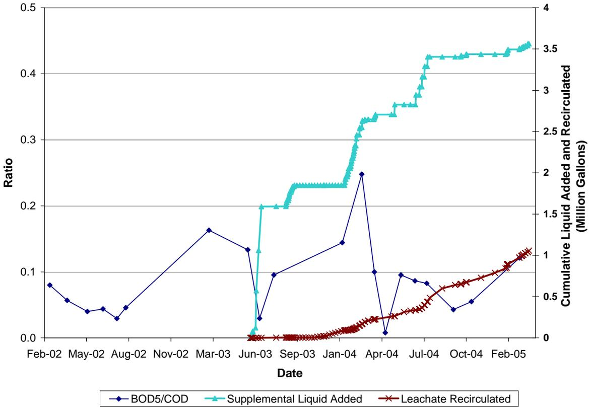
**Figure 11. West-side cell – BOD<sub>5</sub>/COD ratio**
