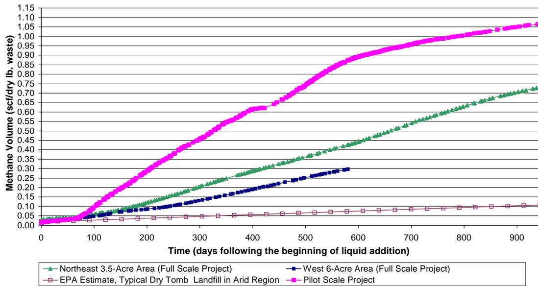
**Figure ES-1. Comparisons among normalized methane production for conventional (brown), Yolo pilot-scale (magenta), northeast (green), and west (blue) accelerated anaerobic composting cells. Note enhancement of methane in pilot-scale, northeast, and west side versus conventional operation.**
