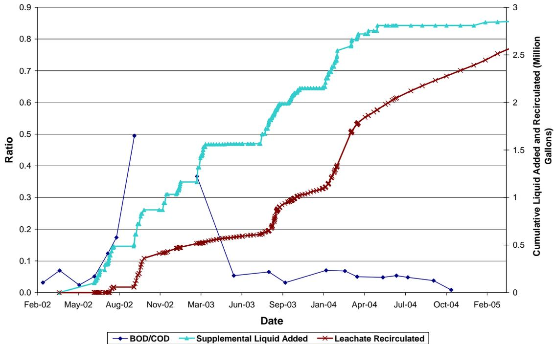
**Figure 10. Northeast cell – BOD<sub>5</sub>/COD over time**
