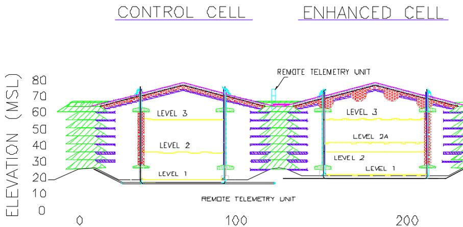
**Detail 3. Cross-section of test cells demonstration project**
