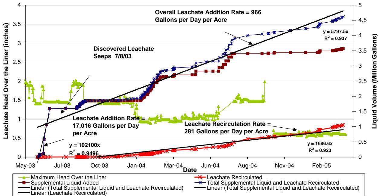
**Figure 8. West-side cell liquid recirculation and addition volumes**
