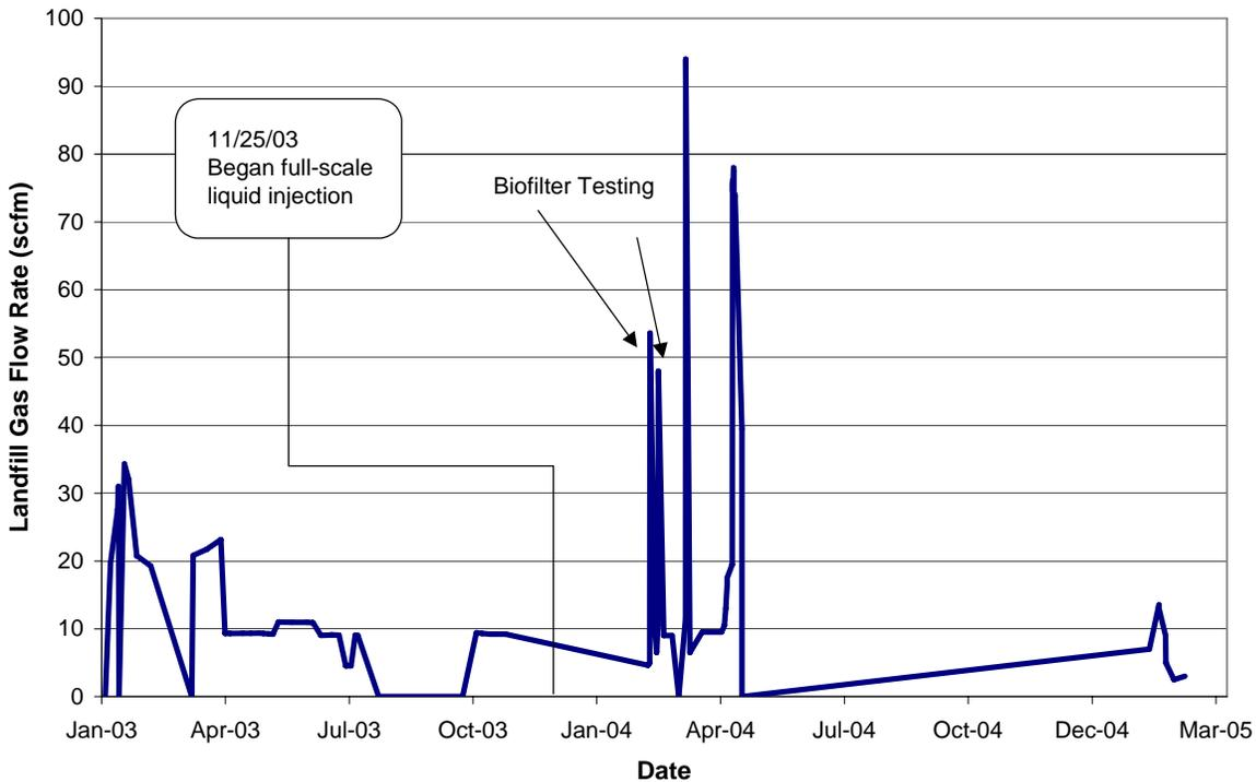
Figure 15. Southeast aerobic cell average daily flow rate
