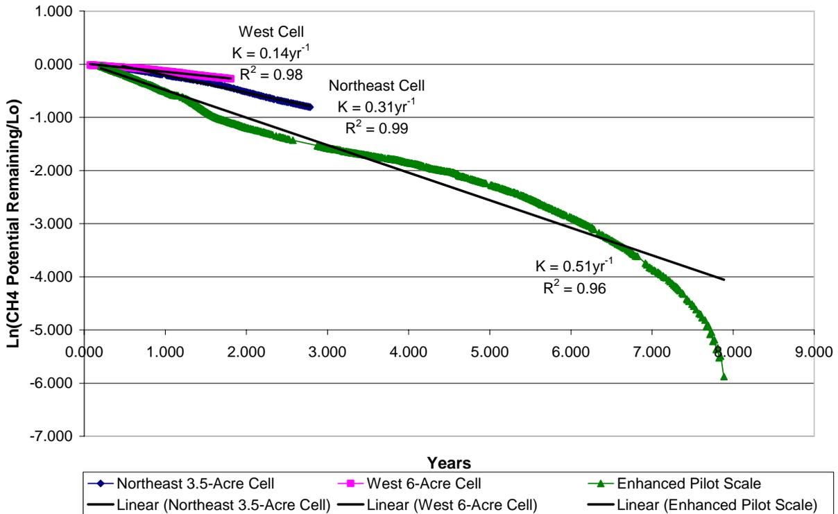
**Figure 19. Calculation of k value for all cells, including previous enhanced cell**
