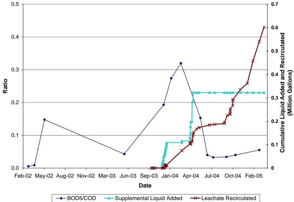
**Figure 12. Southeast aerobic cell - BOD<sub>5</sub>/COD ratio**
