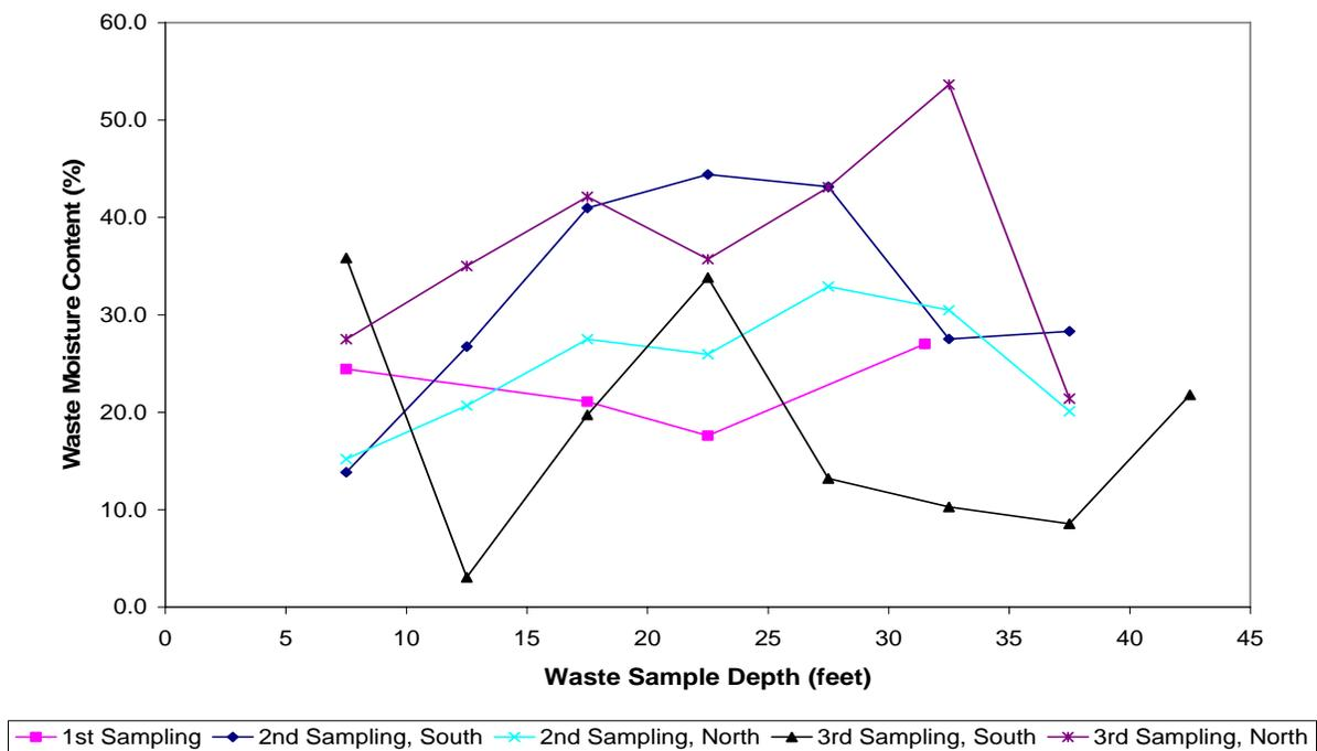
Figure 18. Waste moisture content for the west-side cell
