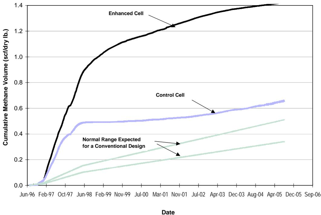
**Figure 2. Cumulated methane recovery of pilot-scale 9000-ton enhanced bioreactor and control. Note the greatly accelerated methane recovery from the enhanced pilot cell relative to conventional and controls.**
