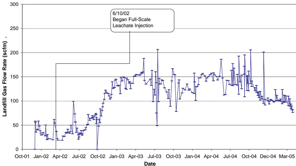
**Figure 13. Northeast cell average daily flow rate**
