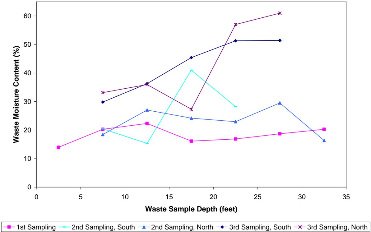
**Figure 17. Waste moisture content for the northeast cell**
